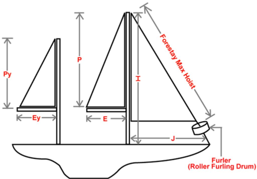
Headsails (Spinnakers require I and J measurements): Attach a tape measure to the jib halyard (or top swivel of the furler) and hoist to the maximum. Measure to the deck sheer line for the I measurement. Also measure to the tack attachment point on the bow (or top of furler) for the maximum hoist measurement. Measure from the intersection of the deck and headstay to the front side of the mast for the J measurement.
